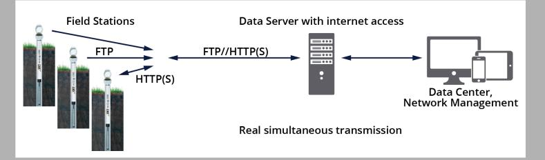
Data is transmitted efficiently in real or near-real time from your monitoring well to your mobile phone or office computer. Transmissions can occur via both HTTP(S) and FTP, of which HTTP(S) allows for two-way communication.
